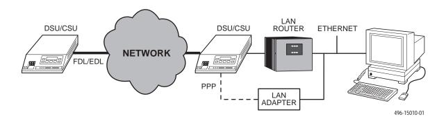
Figure 2-8. Remote Access through FDL/EDL
